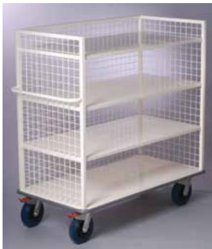
AX 190 Imprest Trolley 1270 x 630 x 1330mm Powder coated finish 4 Shelves - mesh sides and back Full bumper surround / 200mm castors Available with 6 shelves
